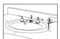
Connect supply line to faucet (finger tight) and carefully bend tubes to engage with the supply shut-off valves. Tighten connections at faucet and shut-off valves for secure seal.
