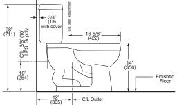
ALL FIXTURE DIMENSIONS ARE NOMINAL AND MAY VARY WITHIN THE RANGE OF TOLERANCES ESTABLISHED BY ASME/ANSI STANDARDS, A112.19.2M. ALL MEASUREMENTS SHOWN ARE SUBJECT TO CHANGE OR CANCELLATION. DIMENSIONS IN PARENTHESES ARE IN MILLIMETERS 25.4 mm = 1 INCH.
