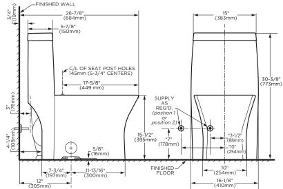
IMPORTANT: Water supply on the wall is required at 3-1/2" (88mm) or 10" (254mm) from centerline of the toilet (see rough-in). First suggested position is hidden behind the toilet. The geometry of the toilet gives space for this installation. The second suggested position is next to the toilet. Between these two positions, the space for the supply between wall and toilet is limited to 4-1/4" (108mm). In this case, check your supply and hose dimensions.
