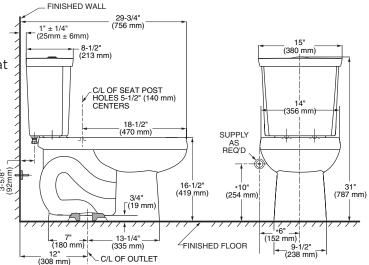
THIS COMBINATION IS DESIGNED TO ROUGH-IN AT A MINIMUM DIMENSION OF 305MM (12") FROM FINISHED WALL TO C/L OF
